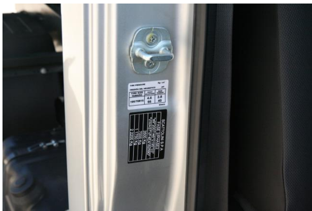
Position of the “2nd Stage Conversion Approval” Decal on Drivers ‘B Pillar.
